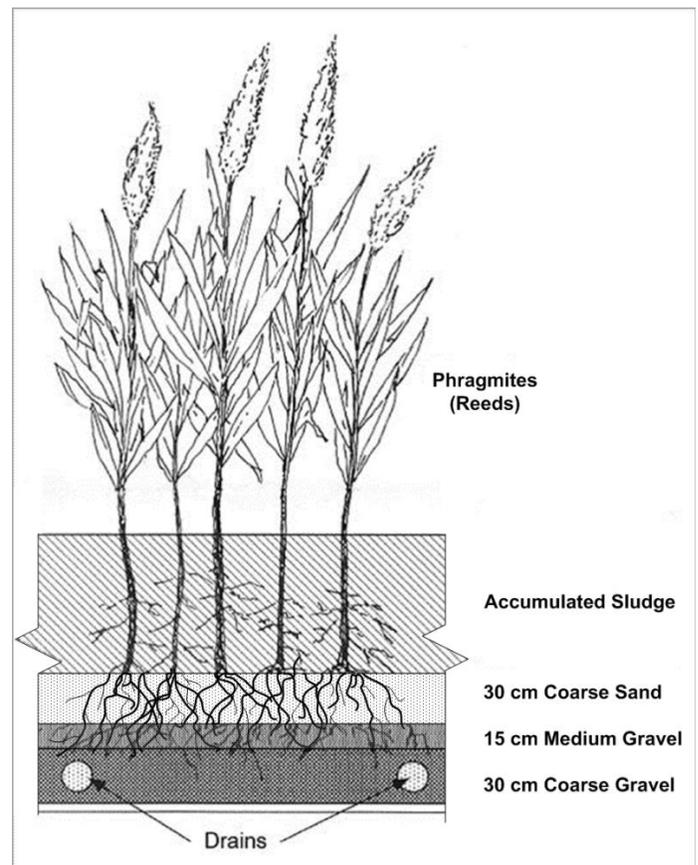
Fig. 1. Schematic of a Reed Bed Filter (Credit: E. Brunet, ORWC)
